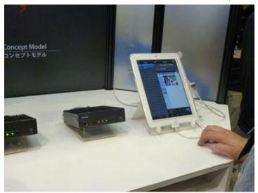
ICOM "concept model" of a black box D-STAR radio with tablet/smartphone user interface:
