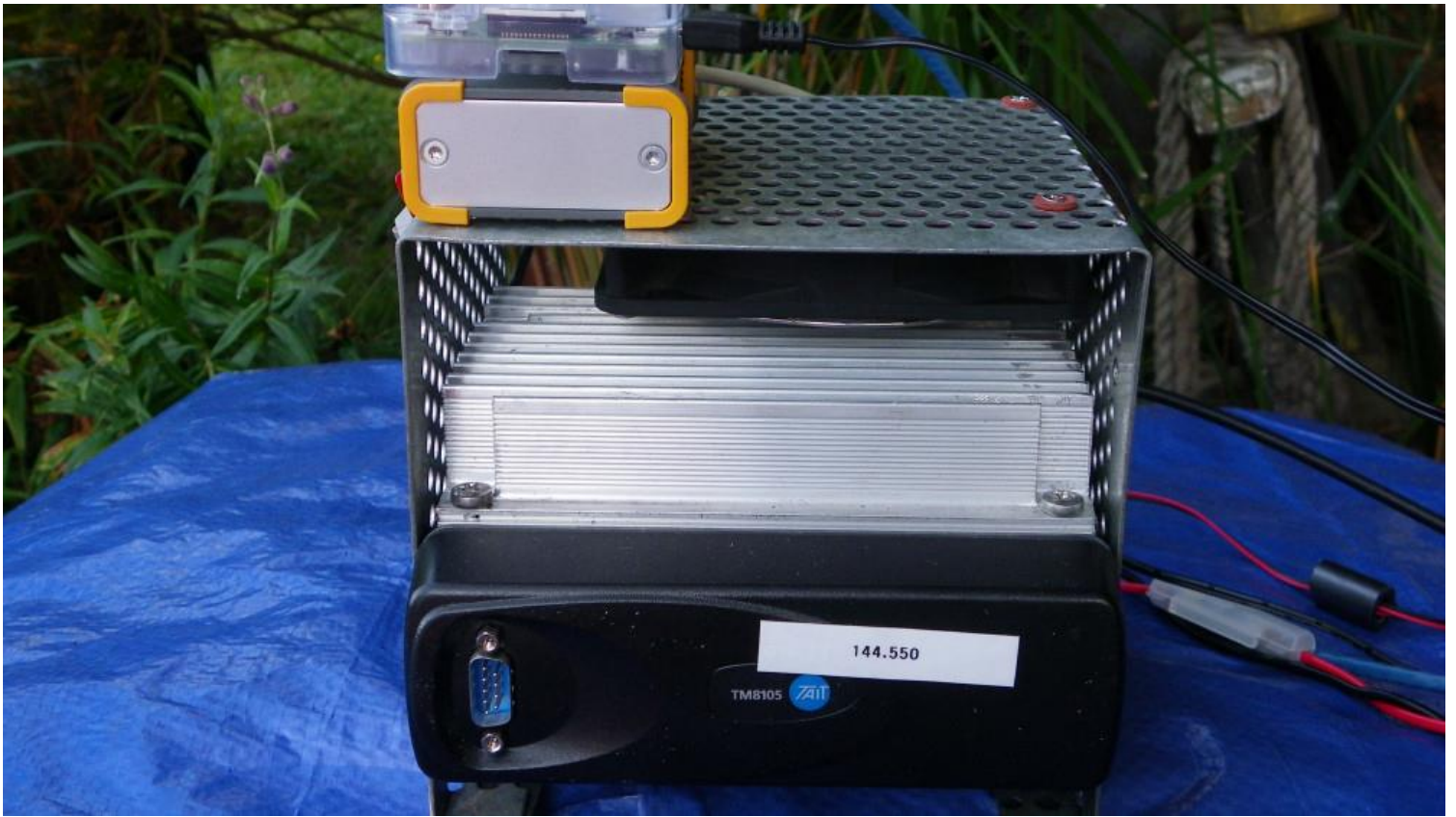
ZL2UDG High Power Hotspot front view. Heatsink and cooling fan used for full time continuous operation.
