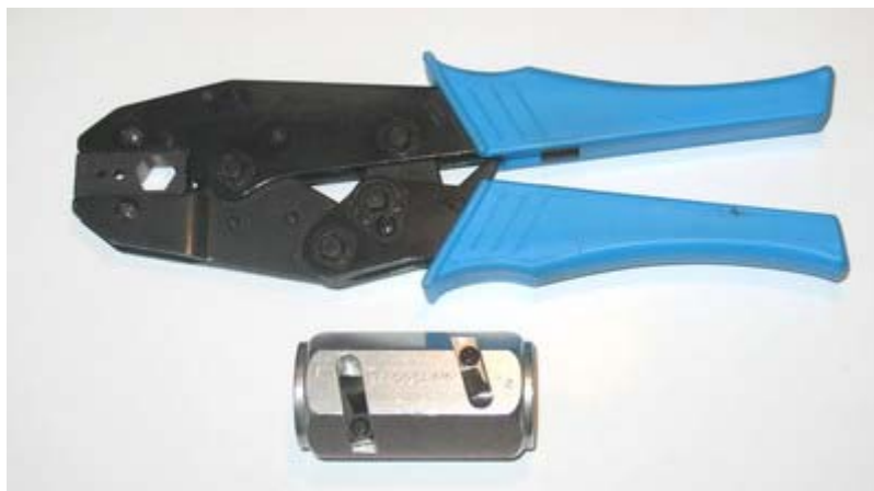
The RF industries crimpers with the .429 die set for LMR-400 size coax and the coax prep tool from Times Microwave.
