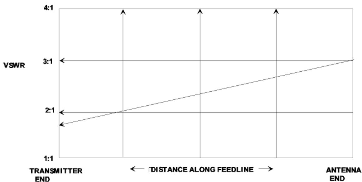
FIGURE 2 EFFECT OF LINE LOSS ON VSWR
