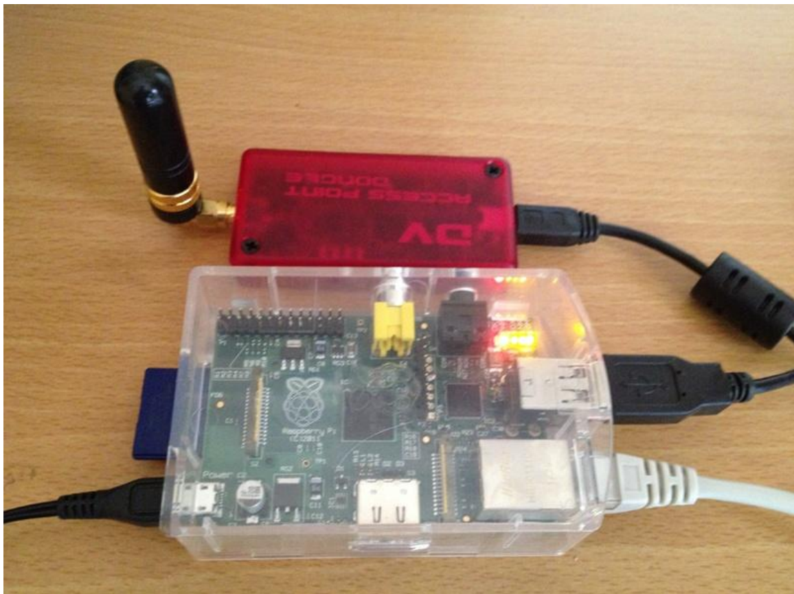
Figure 2: Raspberry Pi – running on ZL2VH Gateway. From the top (going clockwise) is the DVAP (red Box) connected via USB to the Pi, the network cable (beige), power supply (black) and SD Card (blue).
