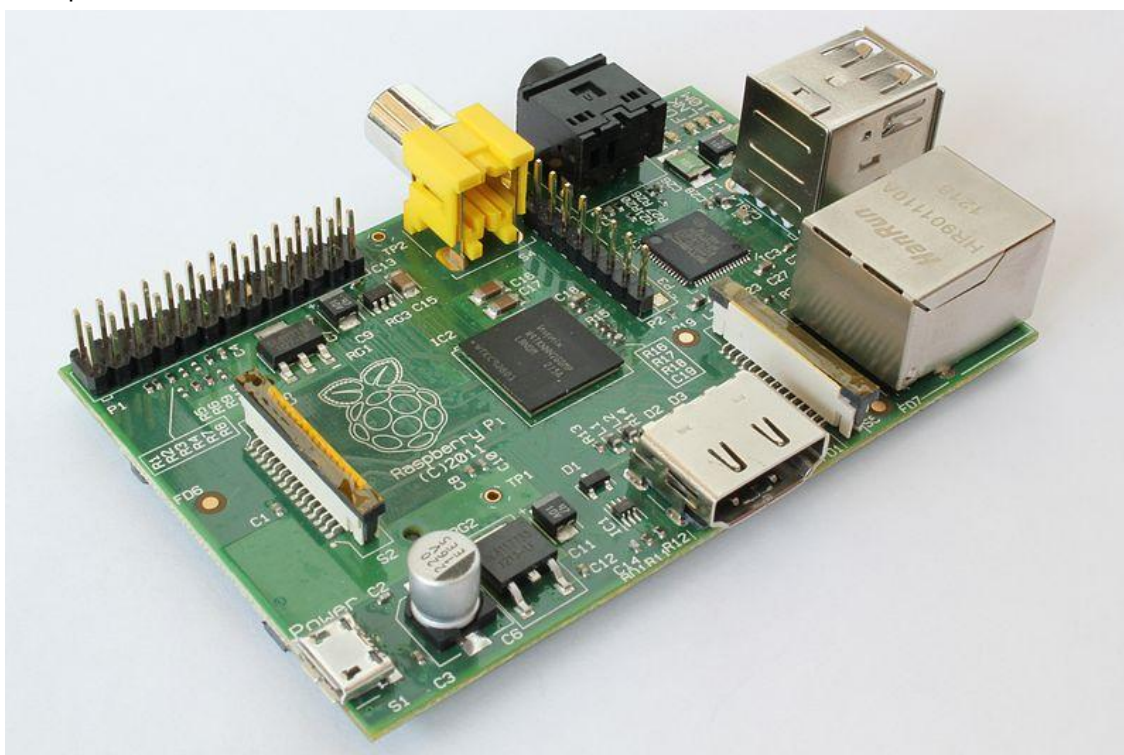
Figure 1: Raspberry Pi - bare circuit board showing the various component sockets.
