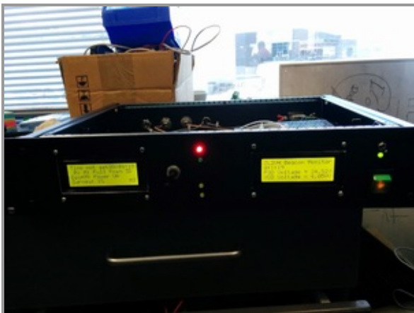
Beacon Controller Front Panel
