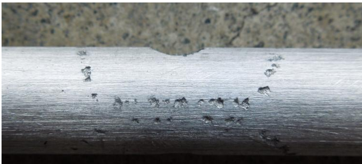
Picture-2: Dipole to boom corrosion pitting.
