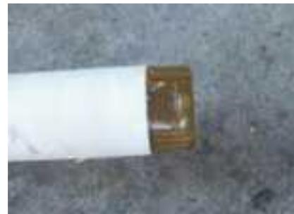
With a high speed cutting disk the resin knob was cut off. The tuning stub could now be adjusted. A sliver plated 3mm diameter wire was used to fine tune the antenna. After tuning a new cap is resin filled and placed back on top. A small 2mm hole is required to release the air as it is pushed on. Tape around the hole until the resin has hardened.
