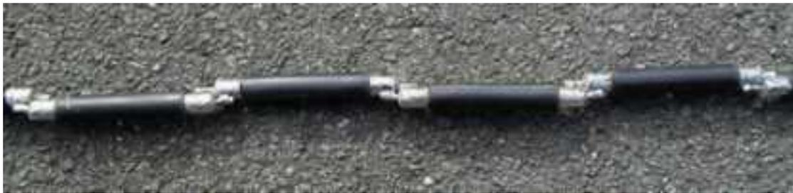
Silver plated wire was wrapped around the connection point for sweat soldering to the copper sleeve balun. A hot plumbers iron was used for a quick solder. This avoids overheating the coax braid and melting the coax dielectric. The antenna is now complete and ready for fitting to the PVC shroud.
