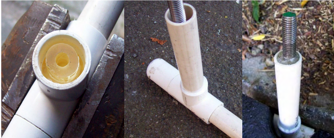
Figure 4: "Plasticast" epoxy high voltage electrical jointing compound poured into the various "T" joints.
