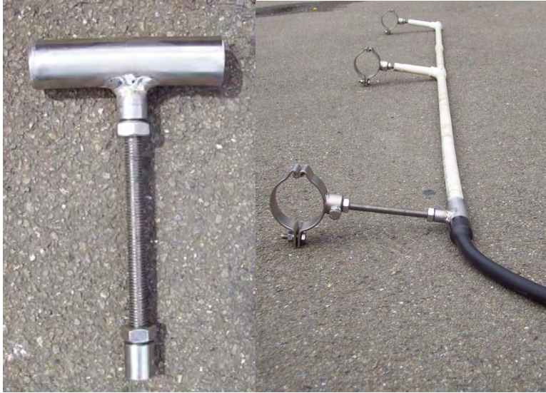
Figure 6: Bottom "T" section on the left. On the right is the completed antenna with the coaxial pigtail attached.
