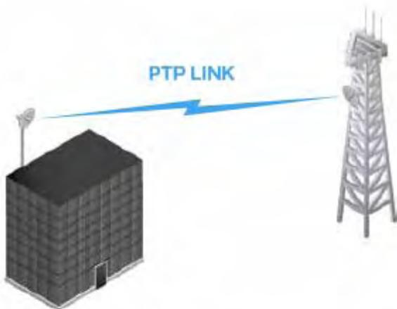
*Using two NanoBridge M to create a powerful, long range, PTP (point to point) link.*
