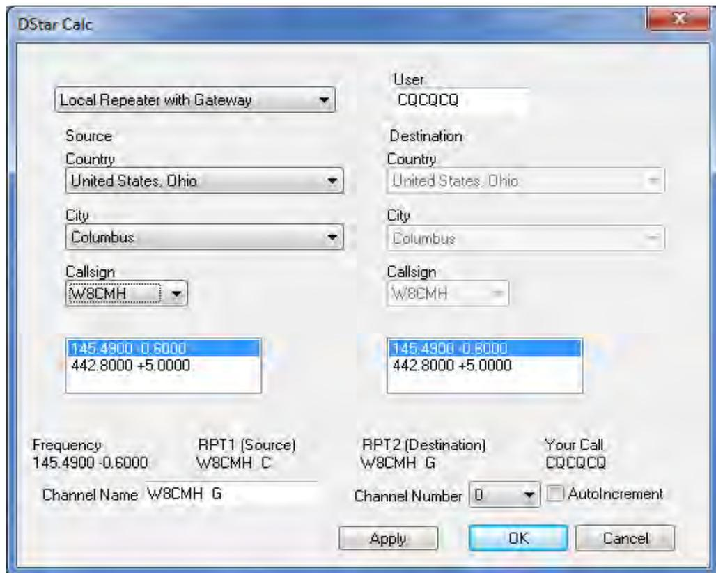
Notice on this page is all the information needed by the radio. Shown above Channel Name is the Frequency setting, RPT1, RPT2 and User (a.k.a. 'UR CALL'). Also W8CMH will be stored in Memory Channel Number 0. Press “OK”.
