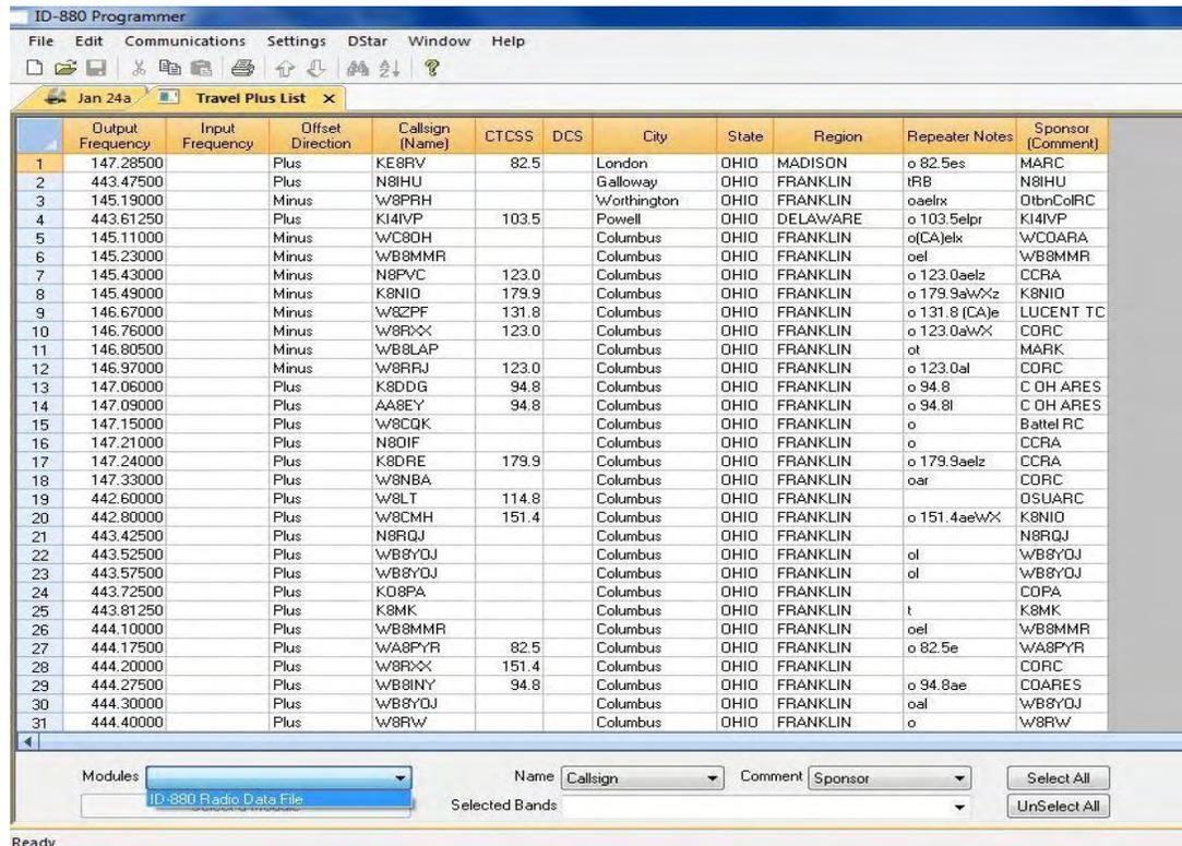
At the lower left of this tab is “Modules”. Click the drop down and ‘ID 880 Radio Data File’ will appear. Next the tab below will have Create Files for ID800. Select this entry.
