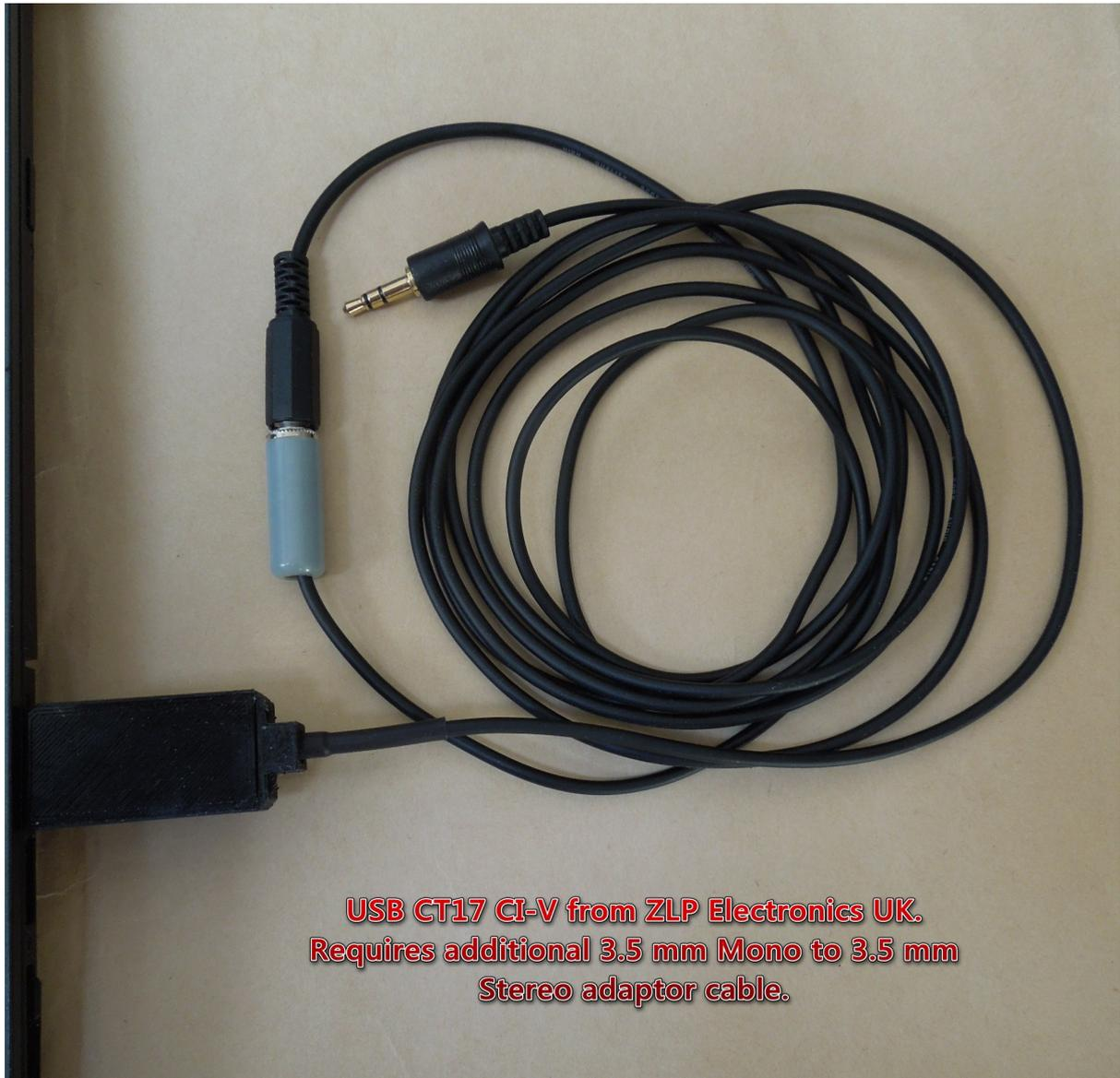
*Figure 2. ID-5100 USB CT17 CI-V modem from ZLP Electronics.*
