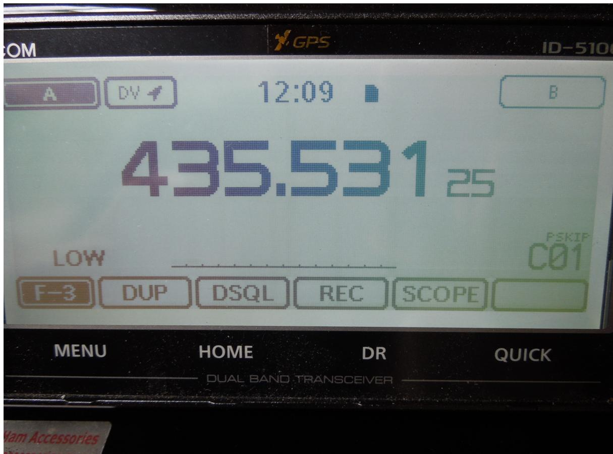
Figure 4. ID-5100 Display 1.25kHz step at AOS tuned to Sparrow DV repeater output.
