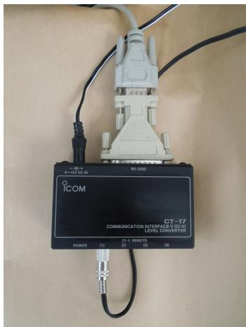
*Figure 1. ID-5100 Icom CT-17 CI-V remote level convertor.*
