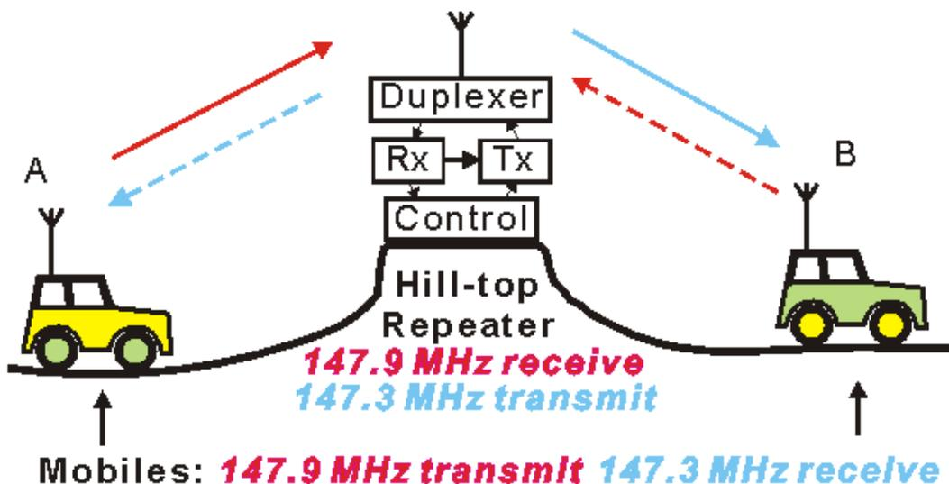
The duplexer allows the transmitter and receiver to both operate at the same time through a single antenna (prevents the repeater transmitter from desensitising the receiver). Have you ever tried to transmit and receive close to someone else who is also using radio transmitters in the same band? Try this and you will see why it is so hard to have simultaneous operation without interference or desensitisation.
