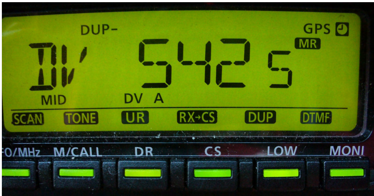
Figure 6: ICOM ID-880H display showing the GPS top right (indicates the GPS Antenna has a satellite lock). "DV A" appears when GPS transmission or GPS-A transmission is selected in the DV mode.
