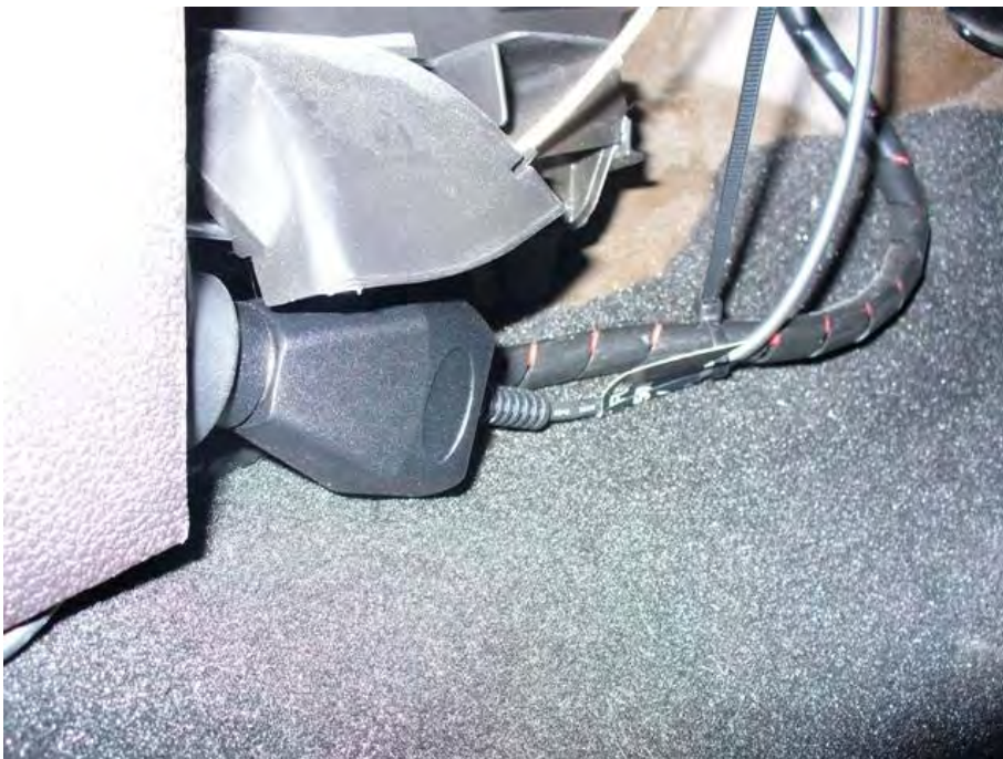
Figure 8: GPS antenna power connector. This cigarette lighter adaptor connects to a Y adaptor from the main socket in the centre console of the vehicle. The cabling is well out of the way travelling across the dashboard under the steering column.
