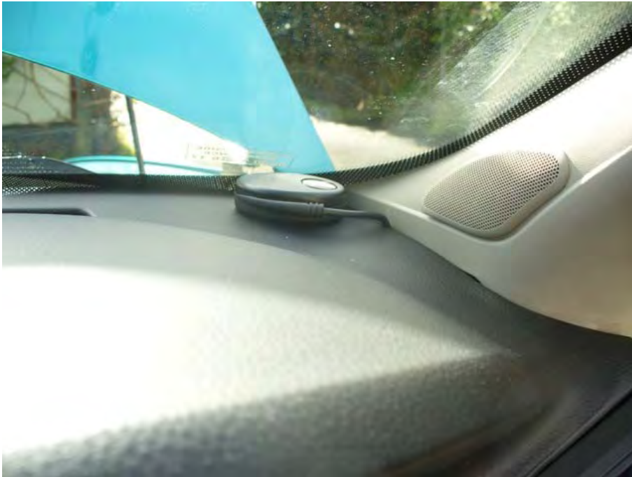
Figure 7: GPS antenna as viewed from driver's seat, with wiring going into the A pillar.
