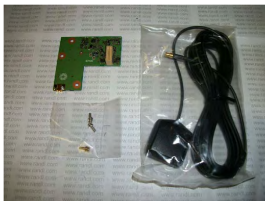
Figure 2: ICOM UT-123 D-Star board and GPS Antenna
