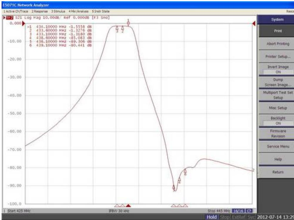
RX pass 433.6 MHz return loss (SWR) -24 db.
