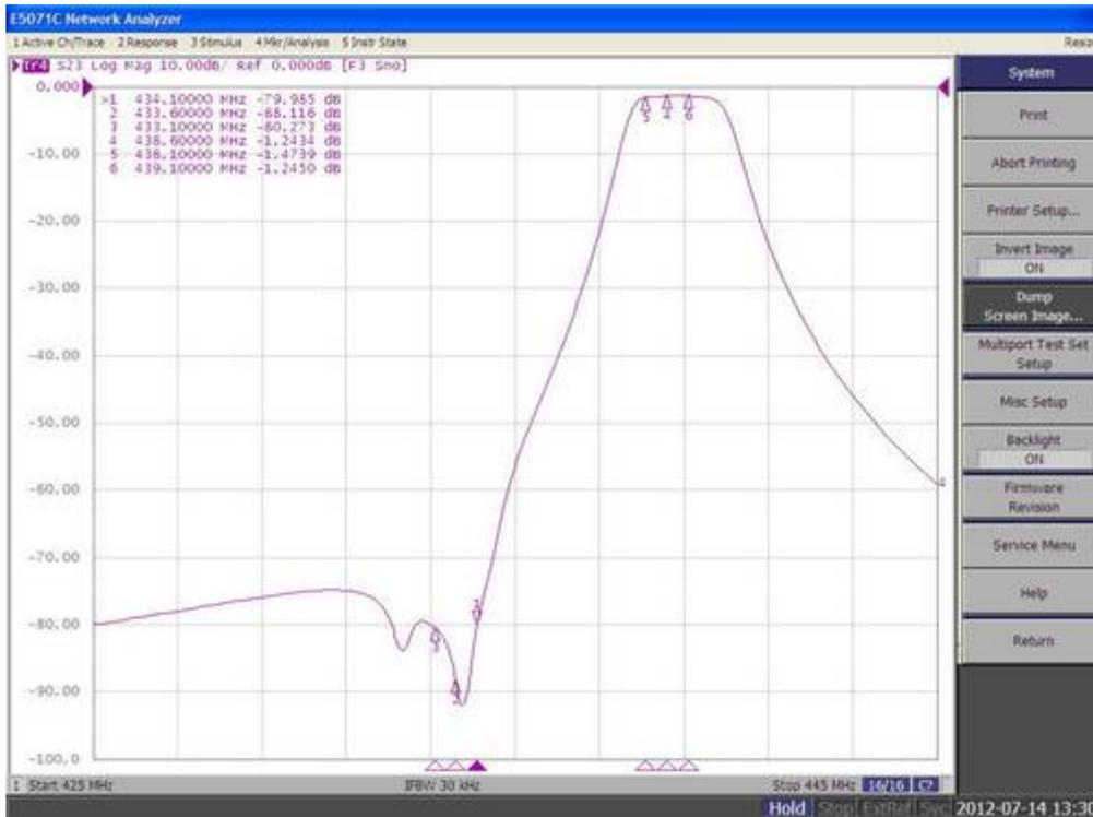
TX pass 438.6 MHz return loss (SWR) -28 db.
